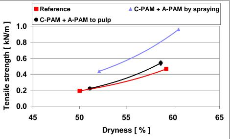
Adding polymers to pulp suspension resulted as lower adsorption of polymers and impaired formation of the sheets (compared to spray application trial point)
