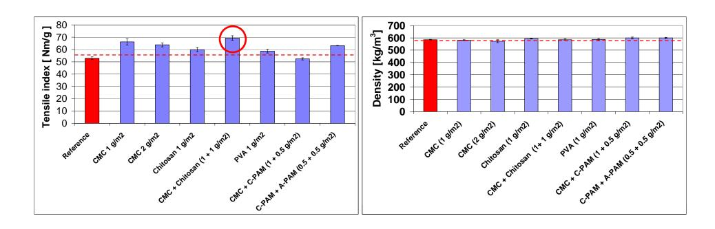
Biggest increase in dry paper tensile strength was obtained with sequential addition of CMC and chitosan
