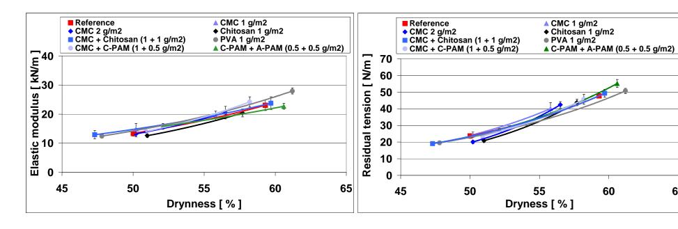
It seems likely that different polymers increased strength of fiber-fiber contacts, but had only minor if any effect on the readiness of fiber segments to carry load
